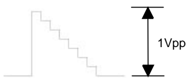
Fig. 14 Signal RGB Pins 1, 3, and 5 of connector P0PC
