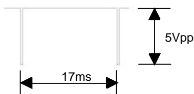
Fig. 18 Vertical Sync Signals TP5854
