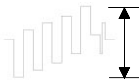
Fig. 20 Signal Pb Pin 3 of Connector P0YU ; 1Vpp
