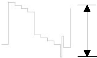
Fig. 19 Signal Y Pins 1 of Connector P0YU ; 1.3Vpp
