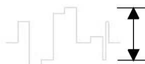
Fig. 21 Signal Pr Pin 5 of Connector P0YU ; 1Vpp
